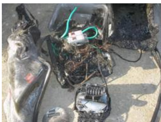
Meter destroyed during attempt to tap into coaxial cable
